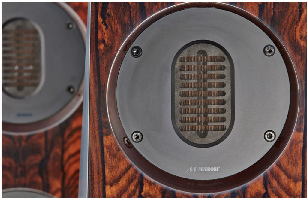
*One can clearly see the folded diaphragm of the AMT tweeter. When in action, the motion is from like that of an accordion*
